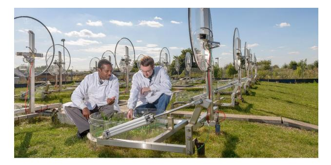
The soil monoliths are 0.8 m in diameter and 1 m deep, enough to be representative of field soil conditions. Each is equipped with systems for controlling moisture and temperature of the soil. Gases emitted from the surface can be monitored and dissolved solutes passing out of the bottom, temperature, moisture and solution at different depths are measured
