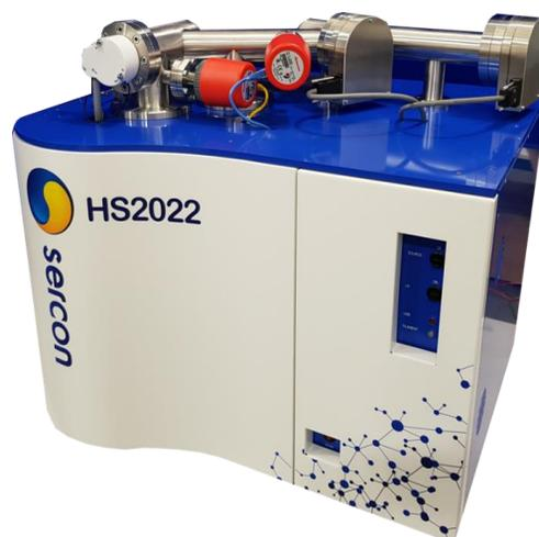
Figure 2 The Sercon HS2022, the world's most sensitive small radius IRMS
