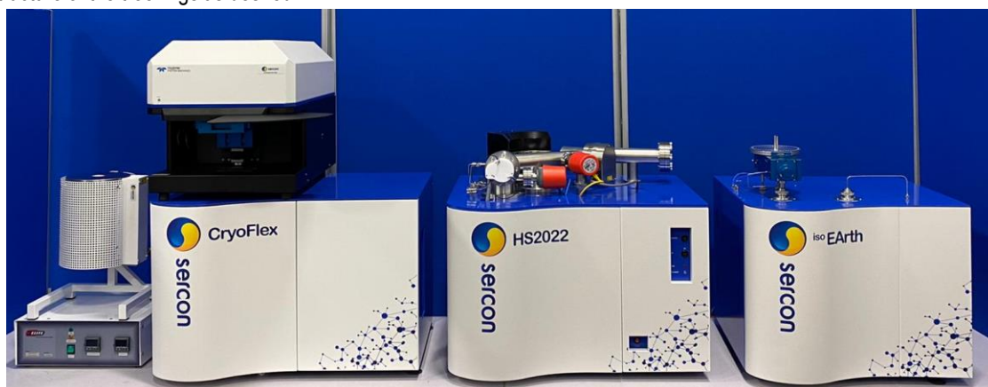
Picture 2 The Sercon LA – IRMS system with Teledyne laser system.
